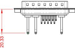
POWER/CO-AX CONTACT RATING:10A (CURRENT)(IF PRESENT)SIGNAL CONTACT CURRENT RATING:5A PER CONTACTSIGNAL CONTACT RESISTANCE:10mΩ MAX.INSULATOR RESISTANCE:5000MΩ min.
