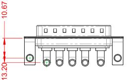
40A (CURRENT) **POWER/CO-AX CONTACT RATING:** (IF PRESENT) SIGNAL CONTACT CURRENT RATING: 5A PER CONTACT SIGNAL CONTACT RESISTANCE:  $10m\Omega$  MAX.
