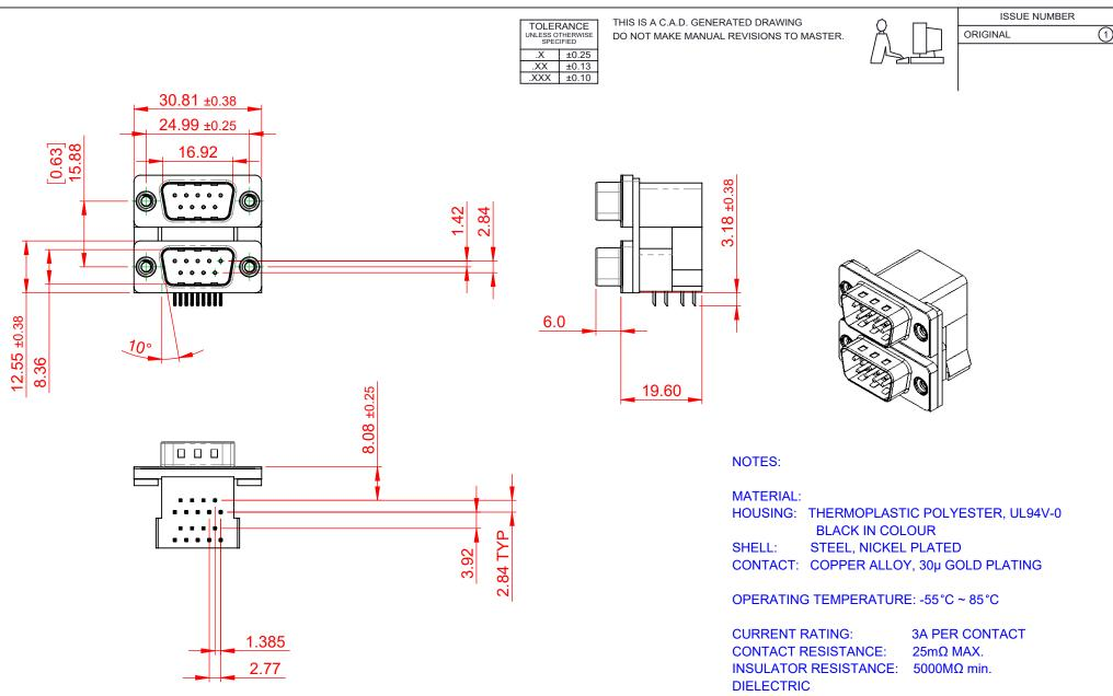
WITHSTANDING VOLTAGE: 1000V AC rms
