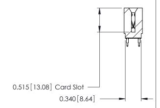
ACAD REFERENCE NO. 746 Series Ultra-Mate Card Edge Connector - Press Fit DRAWN: J.LEE Part Number: 746-066-560-201 CHECKED: **EDAC INC** SCALE: THESE DRAWINGS AND SPECIFICATIONS ARE THE PROPERTY OF EDAC INC.,AND TORONTO, ONTARIO SHALL NOT BE REPRODUCED, OR COPIED DRAWING NUMBER CANADA OR USED AS THE BASIS FOR THE 746-ENG MASTER MANUFACTURE OR SALE OF APPARATUS YOUR CONNECTION TO QUALITY & SERVICE WITHOUT WRITTEN PERMISSION.
