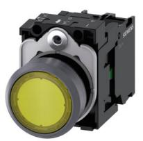
Illuminated pushbutton, 22 mm, round, plastic with metal front ring, yellow, pushbutton, flat, momentary contact type, with holder, 1NO, LED module with integrated LED 110 V AC, screw terminal, with laser labeling, inscription or symbol Customer-specific selection with SIRIUS ACT configurator (CIN)
