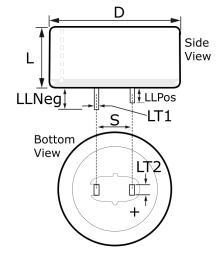
General InformationSeriesFTDescriptionRadial Cylindrical Double Layer CapacitorRoHSYesAEC-Q200NoComponent Weight10 gMiscellaneousDischargeValue = 1.3 F.
