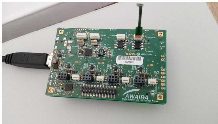
Figure 4 - Connecting NanEye RS to the NANOUSB3 board.
