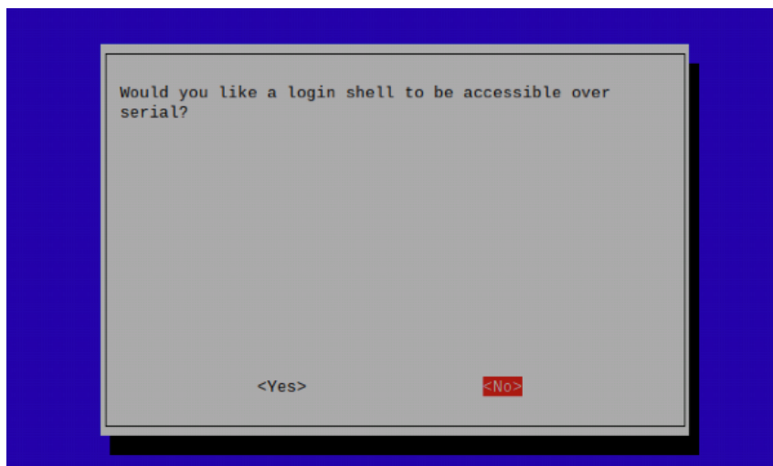
Figure 4. Configuring the serial connection to the Raspberry Pi Build HAT using raspi-config.
