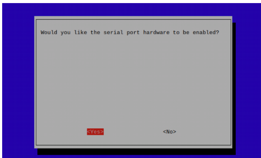
Figure 5. Configuring the serial connection to the Raspberry Pi Build HAT using raspi-config.
