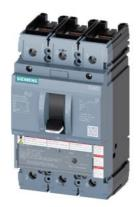
circuit breaker 3VA5 UL frame 250 breaking capacity class C 100kA @ 480 V 3-pole, line protection TM230, FTAM, In=90A overload protection Ir=90A fixed short-circuit protection li=5...10 x In cable connection on both sides
