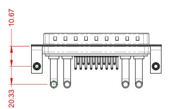
**OPERATING TEMPERATURE:** -55°C ~ 125°C 40A (CURRENT) POWER/CO-AX CONTACT RATING: (IF PRESENT) SIGNAL CONTACT CURRENT RATING: 5A PER CONTACT SIGNAL CONTACT RESISTANCE:  $10m\Omega$  MAX. **INSULATOR RESISTANCE:** 5000MΩ min. DIELECTRIC
