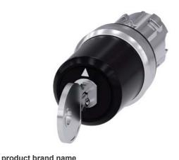
key-operated switch Siemens, 22 mm, round, metal, shiny, lock number SSG10, with 2 keys, 3 switch positions I-O-II, latching, actuating angle 2x45°, 10:30h/12h/13:30h, key removal I+II, with laser labeling, inscription or symbol customer-specific selection with SIRIUS ACT configurator (CIN)
