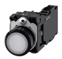
Illuminated pushbutton, 22 mm, round, plastic, white, pushbutton, flat, momentary contact type, with holder, 1 NO+1 NC, LED module with integrated LED 110 V AC, screw terminal, with laser labeling, upper case and lower case, Always upper case at the beginning of the word
