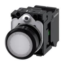
Illuminated pushbutton, 22 mm, round, plastic, white, pushbutton, flat, momentary contact type, with holder, 1NO, LED module with integrated LED 230 V AC, spring-type terminal, with laser labeling, upper case and lower case, always upper case at beginning of line
