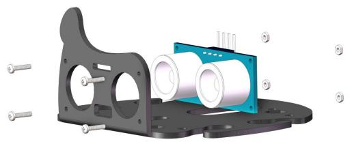
Use a M3\*5 screw to secure the M3\*8 Bi-pass Copper Standoff post on No. 1 board.
