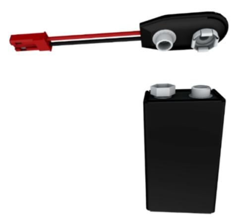
And connect the battery cable to the expansion board.
