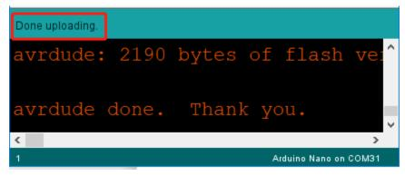
**Note:** If the code cannot be uploaded successfully for a long time, Processor needs to be changed to ATmega328P (Old Bootloader).
