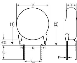
(1) - Coating on lead shall not extend below this line. (2) - Point of support on printed cardboard.
