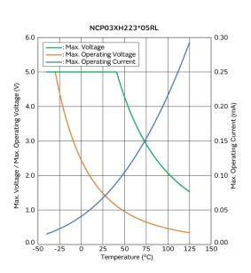
Max. Voltage, Max. Operating Voltage/Current Reduction Curve
