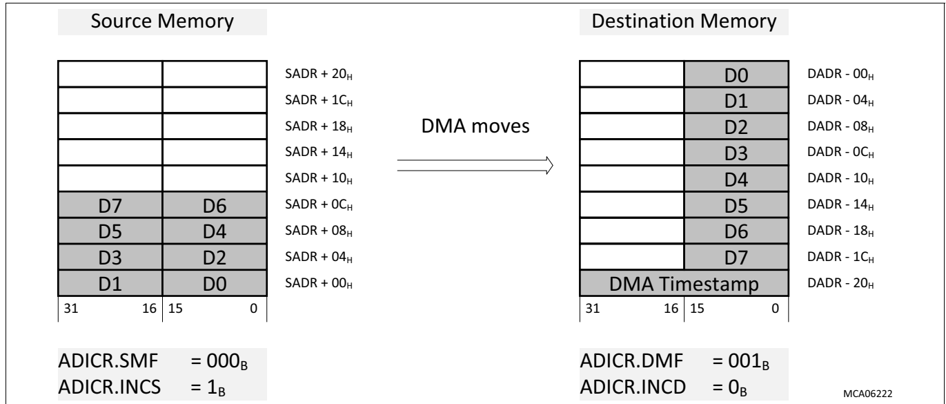
Figure 208 Decrementing Destination Address: DMA Timestamp appended below DMA Write Move Data
