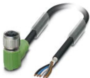
Sensor/actuator cable, 5-position, PUR halogen-free, black-gray RAL 7021, shielded, free cable end, on Socket angled M12 SPEEDCON, A-coded, cable length: 5 m
