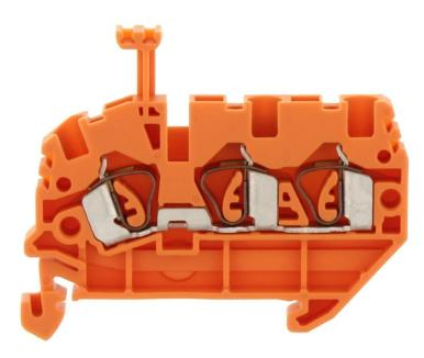
Feed-through terminal, Tension-spring connection, Mounting type: Mounting rail TS 35/7.5, Rated cross-section: 2.5 mm<sup>2</sup>, Width: 5.1 mm, Colour: Orange
