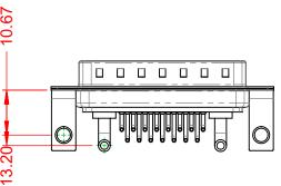
20A (CURRENT) **POWER/CO-AX CONTACT RATING:** (IF PRESENT) SIGNAL CONTACT CURRENT RATING: 5A PER CONTACT SIGNAL CONTACT RESISTANCE:  $10m\Omega$  MAX.
