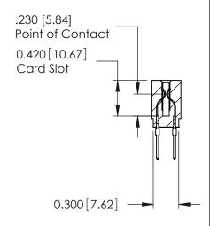
725 Series Ultra-Mate Card Edge Connector - Press Fit ACAD REFERENCE NOSECTION SARA
