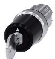
key-operated switch Siemens, 22 mm, round, metal, shiny, lock number SSG10, with 2 keys, 3 switch positions I>O<II, momentary contact type, actuating angle 2x45°, 10:30h/12h/13:30h, key removal O, with laser labeling, upper case and lower case, always upper case at beginning of line
