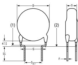
(1) - Coating on lead shall not extend below this line.
