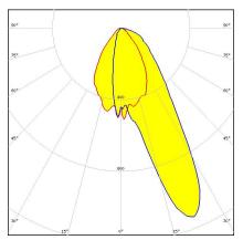
Dimensions: 285.0 mm x 40.0 mm Height: 11.60 mm Asymmetric beam for wall-washing and
