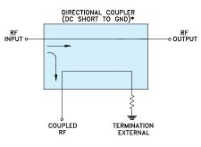
\* ELECTRICAL SCHEMATIC IS FOR DIRECTIONAL COUPLER WITH INTERNAL TRANSFORMER(S) AND EXTERNAL TERMINATION.
