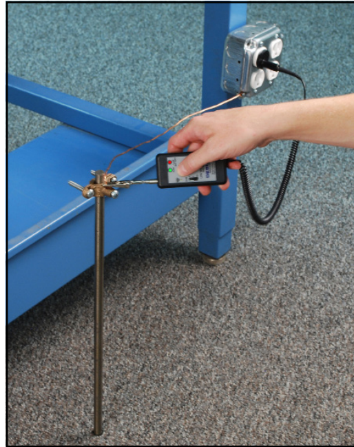
Figure 5. Testing auxiliary ground with the 19249 tester
