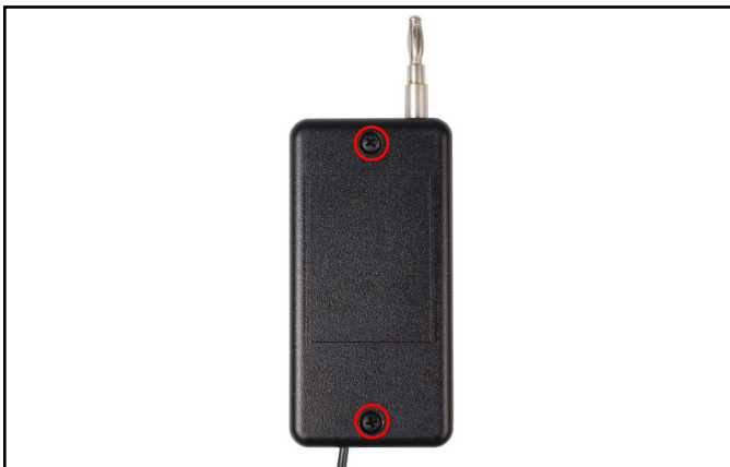
Figure 6. Locating the enclosure screws
