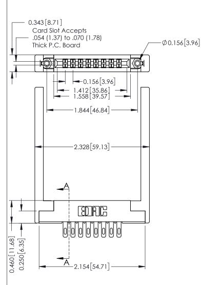
SECTION A-A 0.295 [7.49] Card Slot 0.165[4.19] Point of Contact
