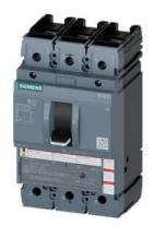
circuit breaker 3VA5 UL frame 250 breaking capacity class M 35kA @ 480 V 3-pole, line protection TM210, FTFM, In=225A overload protection Ir=225A fixed short-circuit protection Ii=10 x In UL489 SB (naval), 50 deg. cel. nut keeper kit on both sides
