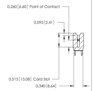
ACAD REFERENCE NO. 746-ENG MASTER 746 Series Ultra-Mate Card Edge Connector - Press Fit DRAWN: J.LEE DATE: AUG 20/09 Part Number: 746-048-520-206 CHECKED: DATE: **EDAC INC** SCALE: SHEET 1 OF 1 THESE DRAWINGS AND SPECIFICATIONS ARE THE PROPERTY OF EDAC INC.,AND TORONTO, ONTARIO SHALL NOT BE REPRODUCED, OR COPIED DRAWING NUMBER CANADA OR USED AS THE BASIS FOR THE 746-ENG MASTER MANUFACTURE OR SALE OF APPARATUS YOUR CONNECTION TO QUALITY & SERVICE WITHOUT WRITTEN PERMISSION.
