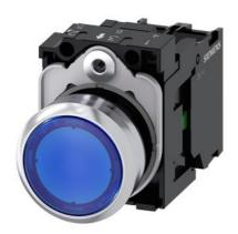
Illuminated pushbutton, 22 mm, round, metal, shiny, blue, pushbutton, flat, momentary contact type, with holder, 1NO, LED module with integrated LED 110 V AC, screw terminal, with laser labeling, lower case
