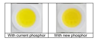
The color spectrum is different between the new phosphor and current phosphor as illustrated below.
