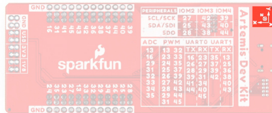
Silk marking the orientation of the accelerometer's axes, in reference to the Artemis Development Kit. (Click to enlarge)
