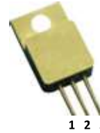
TO – 257 (Isolated Base-plate Hermetic Package)
