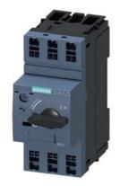
Circuit breaker size S00 for transformer protection A-release 0.14...0.2 A N-release 4.2 A Spring-type terminal Standard switching capacity
