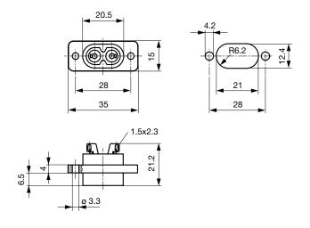
Solder terminals for wires
