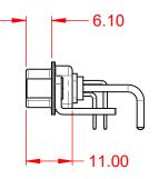
MATERIAL: HOUSING: THERMOPLASTIC POLYESTER, UL94V-0 STEEL, NICKEL PLATED SHELL: CONTACT: COPPER ALLOY, GOLD FLASH PLATED **OPERATING TEMPERATURE:** -55°C ~ 125°C 10A (CURRENT) POWER/CO-AX CONTACT RATING: (IF PRESENT) SIGNAL CONTACT CURRENT RATING: 5A PER CONTACT SIGNAL CONTACT RESISTANCE:
