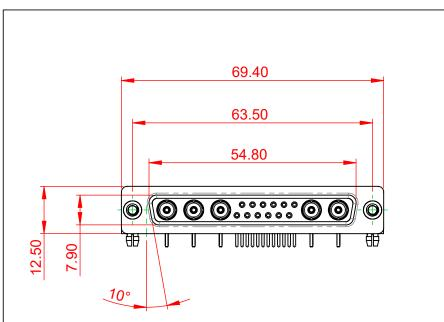
THIS IS A C.A.D. GENERATED DRAWING TOLERANCE UNLESS OTHERWISE SPECIFIED DO NOT MAKE MANUAL REVISIONS TO MASTER. .X ±0.25 .XX ±0.13 .XXX ±0.05
