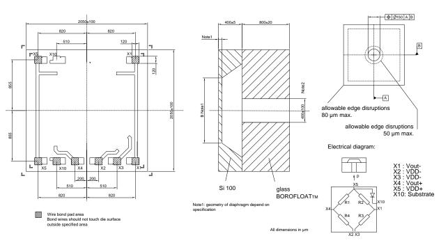
All technical data are defined for pressure application from passive side. Sign of output voltage will change by pressure application from active side.
