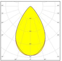
Dimensions: 21.6 mm x 21.6 mm Height: 13.10 mm ~65° wide beam optimized for CREE
