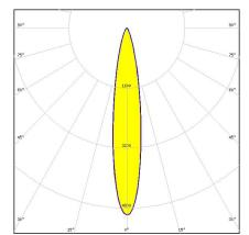
Dimensions: 21.6 mm x 21.6 mm Height: 13.10 mm ~15° diffused spot beam optimized for CREE XP-E. Assembly with white holder, installation tape and
