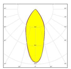
**Dimensions: 21.6 mm x 21.6 mm Height: 13.10 mm** ~65° wide beam. Assembly with thinner white holder, installation tape and location pins.
