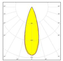
Dimensions: 21.6 mm x 21.6 mm Height: 13.10 mm ~30° medium beam optimized for CREE XP-E. Assembly with black holder and installation tape.
