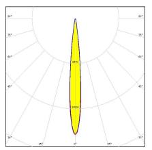
**Dimensions: 21.6 mm x 21.6 mm Height: 13.10 mm** ~11° smooth spot beam optimized for CREE XP-E. Assembly with black holder and installation tape.
