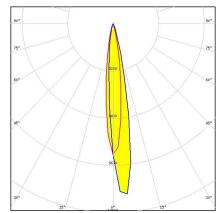
Dimensions: 21.6 mm x 21.6 mm Height: 13.10 mm Asymmetric beam for wall-washing
