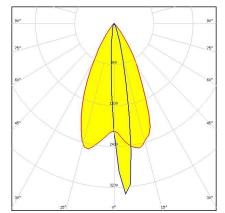
Dimensions: 21.6 mm x 21.6 mm Height: 13.10 mm Asymmetric oval beam for wall-washing. Assembly with thinner white holder, installation tape and location pins.
