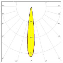
Dimensions: 21.6 mm x 21.6 mm Height: 13.10 mm ~8° spot beam. Assembly with thinner white holder, installation tape
