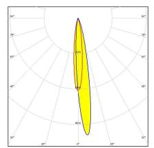
**Dimensions: 21.6 mm x 21.6 mm Height: 13.10 mm** Asymmetric beam for wall-washing. Assembly with thinner white holder, installation tape and location pins.
