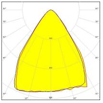
**Dimensions: 21.6 mm x 21.6 mm Height: 13.10 mm** Mini reflector with ~72° wide beam. Assembly with thinner white holder, installation tape and location pins.
