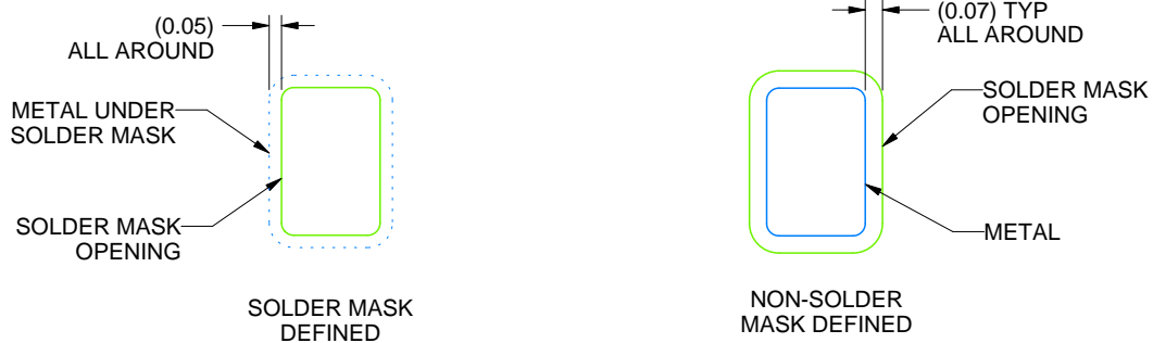
SOLDER MASK DETAIL
