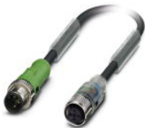
Sensor/actuator cable, 3-position, Variable cable type, Plug straight M12 SPEEDCON, A-coded, on Socket straight M12 SPEEDCON, A-coded, with 2 LEDs, cable length: Free input (0.2 ... 40.0 m)
