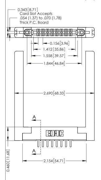
SECTION A-A 0.295[7.49] Card Slot 0.090[2.29] Point of Contact 305 ENG MASTER 305 / 315 / 355 Card Edge Connector DATE: SEPT. 21/09 J.LEE Part Number: 355-016-520-258
