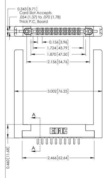
SECTION A-A 0.295[7.49] Card Slot 0.090 [2.29] Point of Contact 305 ENG MASTER 305 / 315 / 355 Card Edge Connector
