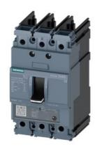
circuit breaker 3VA5 UL frame 125 breaking capacity class H 65kA @ 480V 3-pole, line protection TM230, FTAM, In=35A overload protection Ir=35A fixed short-circuit protection Ii=5...10 x In UL 489 SB (naval), 50° C without connection
