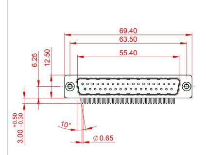
TOLERANCE UNLESS OTHERWISE SPECIFIED XX ± 0.13 XXX ± 0.10 THIS IS A C.A.D. GENERATED DRAWING DO NOT MAKE MANUAL REVISIONS TO MASTER. 11.0 ±0.3 6.10
