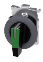
Selector switch, illuminable, 30 mm, round, Metal, matte, green, selector switch, long, front ring for flush installation, 3 switch positions I>O<II, momentary contact type, actuating angle 2x45°, 10:30h/12h/13:30h, Z=50-unit packaging
