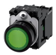
Illuminated pushbutton, 22 mm, round, plastic, green, pushbutton, flat, momentary contact type, with holder, 1NO, LED module with integrated LED 24 V AC/DC, screw terminal, Z=20-unit packaging
