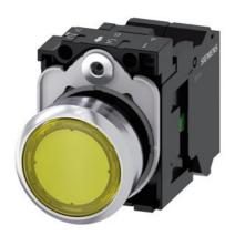
Illuminated pushbutton, 22 mm, round, metal, shiny, yellow, pushbutton, flat, momentary contact type, with holder, 1NO, LED module with integrated LED 24 V AC/DC, spring-type terminal, with laser labeling, lower case
