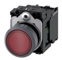
Illuminated pushbutton, 22 mm, round, plastic with metal front ring, red, pushbutton, flat, momentary contact type, with holder, 1NO, LED module with integrated LED 24 V AC/DC, screw terminal, with laser labeling, symbol number according to, ISO 7000 or IEC 60417
