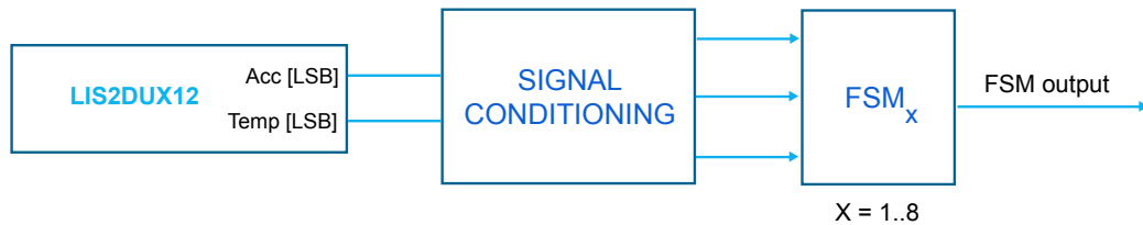
Figure 10. State machine in the LIS2DUX12
